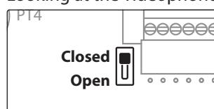
Move the switch to the upper position to enable the BUS termination (**Closed** position, factory setting)
