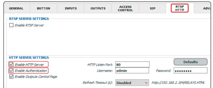
**Fig. 11** Enable Authentication from IPure Wizard software
