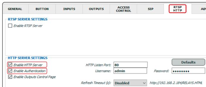
**Fig. 14** Enable Authentication from IPure Wizard software
