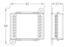
4 Way compact active video distribution box for video door entry systems using balanced video signal.
