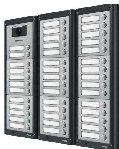
9 modules installation example with 1 video speaker unit and 8 modules 4045/M for 42 total push buttons
