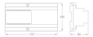
230V input, 13.5Vac 1.6A Max (pulsed) or 13.5Vdc 0.8A continuous (1A pulsed) outputs power supply unit. The power transformer is built in a 9 modules A type DIN box (157 mm) and can be installed on a DIN bar or fixed directly to the wall.
