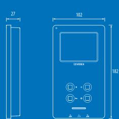
The 6300 series surface mount video monitor with a 3.5" Hi-Res full colour active matrix LCD screen is designed primarily for low and high-rise private developments and individual houses where an attractive and low cost functional videophone is desirable.
