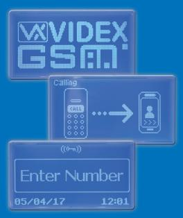
Blue back-lit 128x64 pixel graphical LCD display with call progress indication and integrated voice annunciation.
