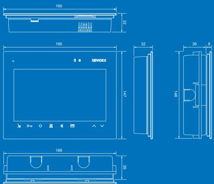
The 7" video monitor with an 800x480 pixel resolution full colour active matrix LCD screen is designed primarily for low and high-rise private developments and individual houses where an attractive functional video monitor is desirable.
